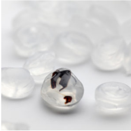
Testable pellets/polymers with defects
