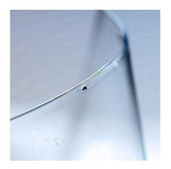
Extruded polymerfilm with visible defects
