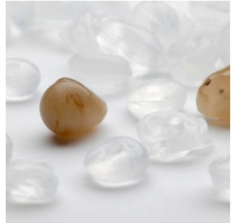
**Testable pellets/polymers with defects**
