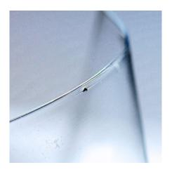
Extruded polymerfilm with visible defects
