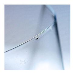
Extruded polymerfilm with visible defects
