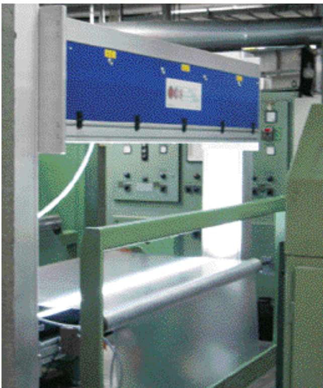
Fig. 2. Closed inspection bridge
