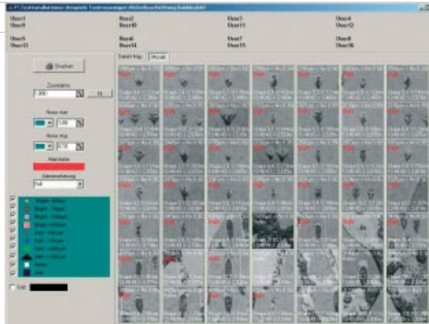
Errors must be classified once by the operator on the basis photos; afterwards the system recognises the errors automatically
