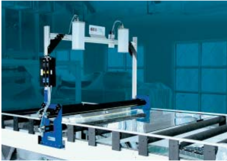
Fig. 2. Open inspection bridge to inspect polycarbonate sheet
