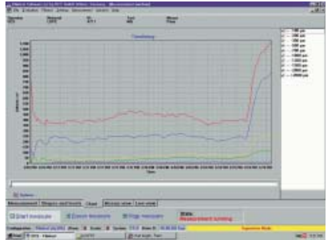
Fig. 2. Statistical representation of the defect rate, e.g. gel content, help to recognise production trends at an early stage
